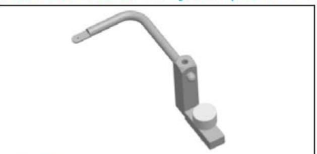
The electrode zero adjuster is used to set the electrode during the experiment. In the vertical direction, the reference point is 30 mm higher than the ear bar reference point, the ear bars are used with 68000 series stereotaxic instruments.
