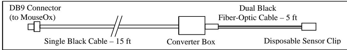
1] Connect the DB9 Connector (9-pin connector) on the end of the thin black cable to the MouseOx® Control Box. Be sure that the MouseOx® software is not running when you do this.
