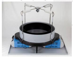
A stand positioned over the device holds the camera and 4 dual (visible/I.R. lights)
