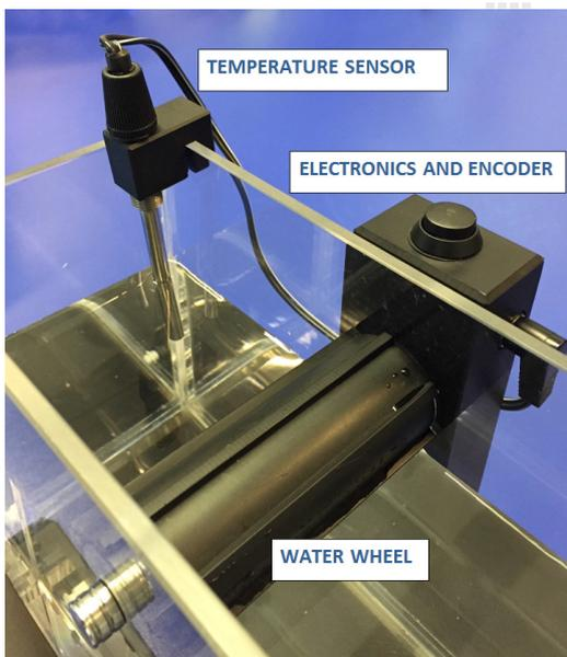
The water wheel has a diam. of 3.5cm and is 8cm wide; six 0.5cm paddles are evenly positioned on the wheel surface.
