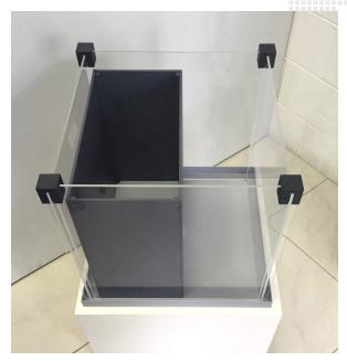
The Mouse Cage is made of a Start Box (dark chamber) I.D. 42x20x35(h)cm and a Test Box (light chamber) with the same dimensions.
